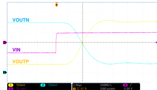
Figure 8-4. Step Response of the AMC1202
