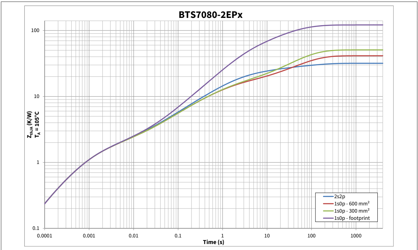
Figure 9 Typical Thermal Impedance. PCB setup according Chapter 4.4.1
