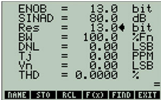
Figure 4. The ENOB Calculator determined that 13 bits of resolution are required in our example.
