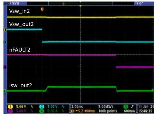
Figure 31. Power Switch2 Current Limit Operation
