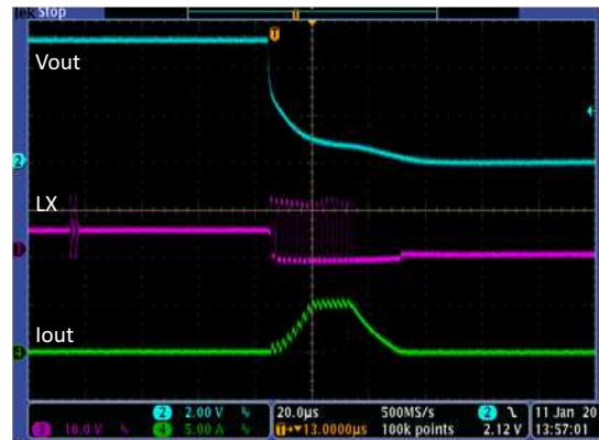
Figure 21. Zoom in Buck Output Hard-Short Response
