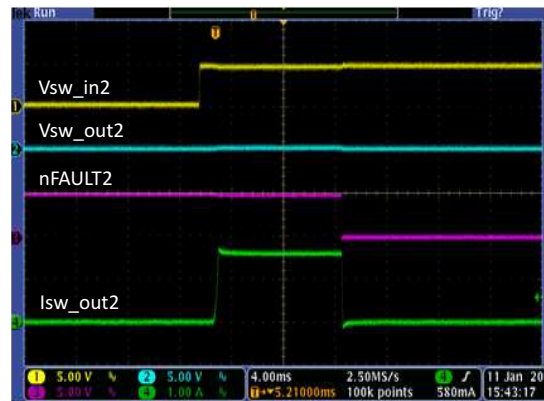
Figure 29. Power Switch2 Enable Into Short Circuit
