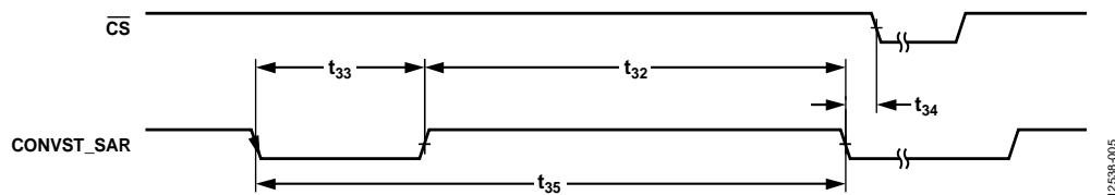
Figure 5. SAR ADC Timing Diagram
