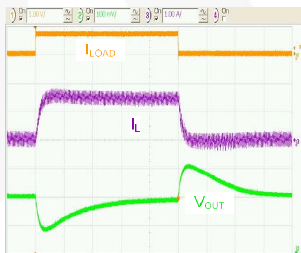
Figure 7. Load Transient Response, 3.3V OUT (100mA to 1500mA, 20μs/div)
