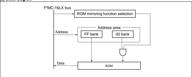
Note: Do not access to ROM mirroring function selection register in the middle of the operation of the address 008000H to 00FFFFH.
