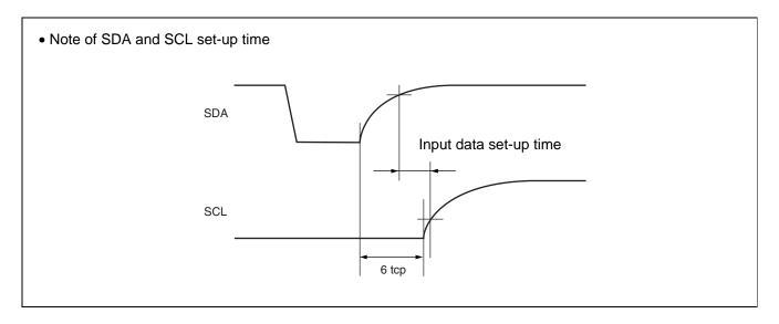
Note: The rating of the input data set-up time in the device connected to the bus cannot be satisfied depending on the load capacitance or pull-up resistor.
